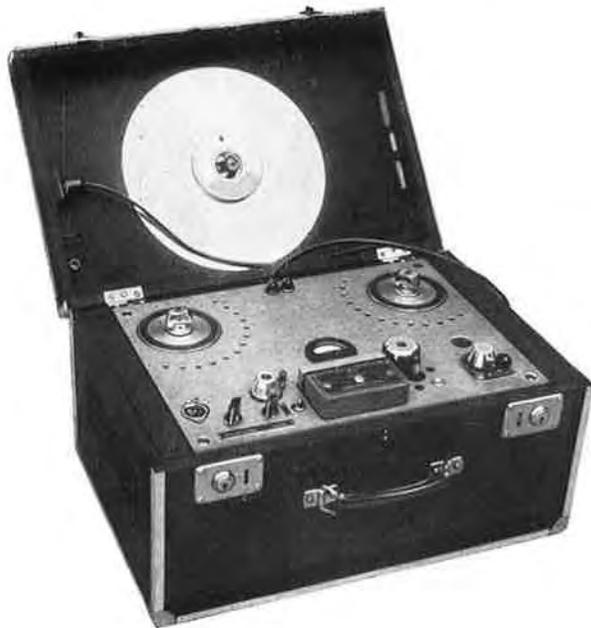
The picture shows a type MTG 9-54 AW/K portable Tape Recording Machine for recording and playback. The type AWL/K Tape Recorder contains an additional 4 watt power amplifier, mounted into the carrying case, and a monitor speaker on the right hand side of the case. The type MTG 9 W/K Playback Machine is designed for playback only and therefore does not have the microphone input connector, the VU-meter, the record-switch and control light.
